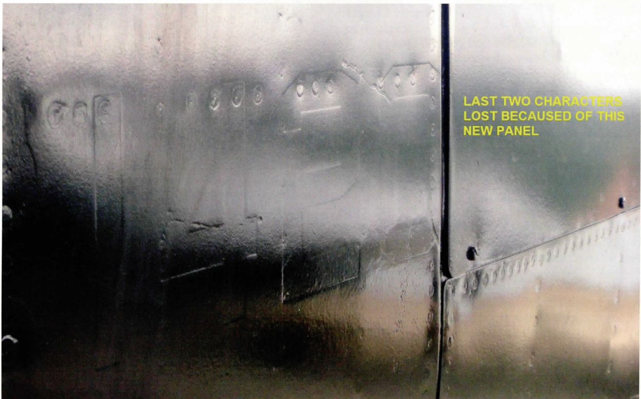
The first four numbers of serial 142072 can be clearly seen under the paint. The last two numbers are lost because a new plate has been fitted.
