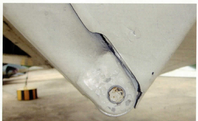
Undamaged outboard flap hinge.
