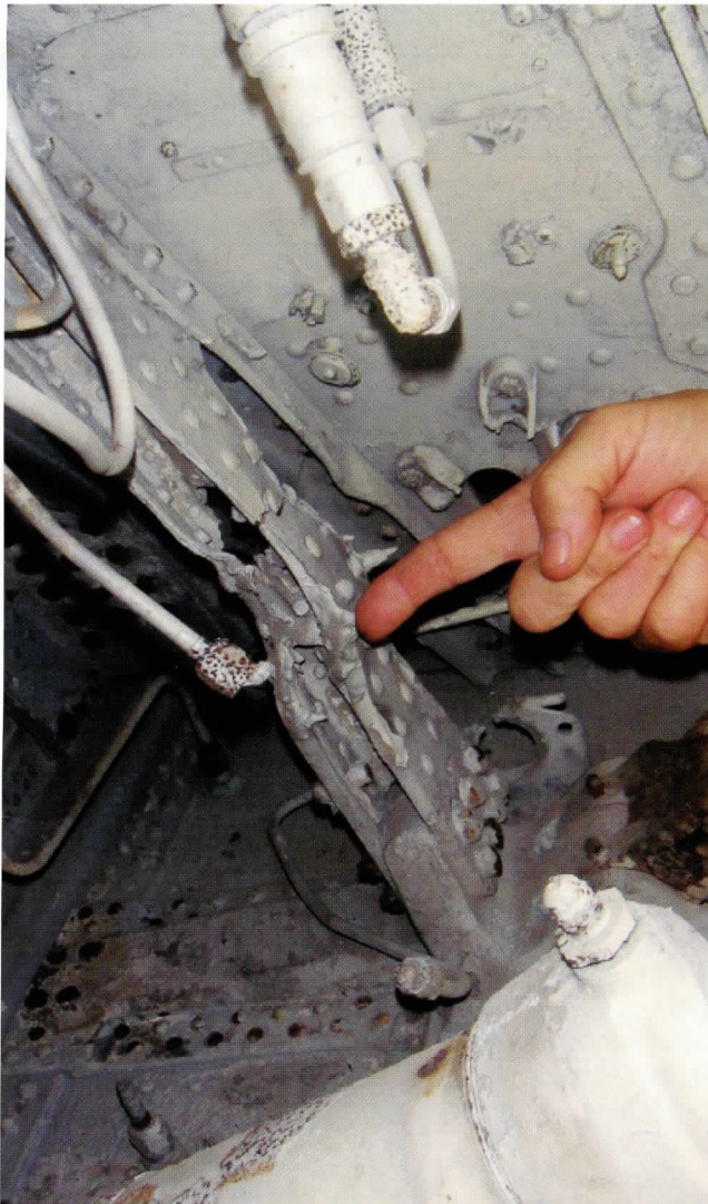
Above left and right: Damage to starboard wheel-well caused by belly-landing.
